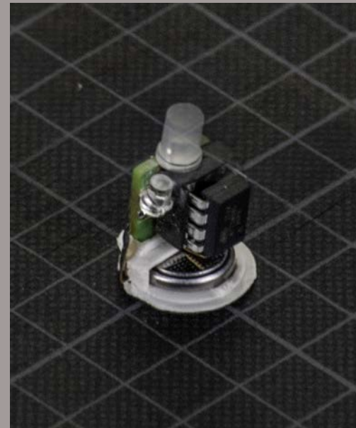
An assembled unit placed on the battery holder
