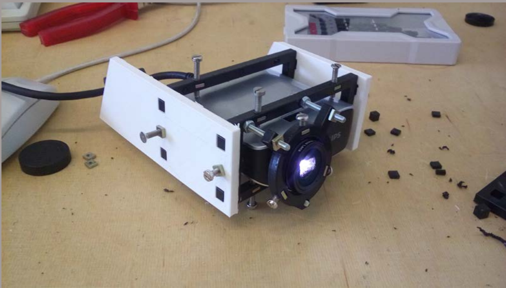
First tests of building a mount for a fish eye lens on a pico projector
