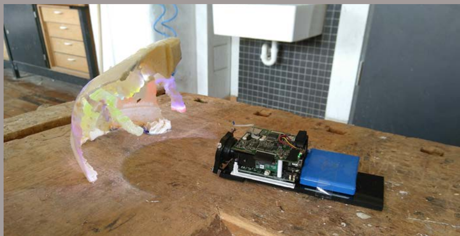
To find the material with the best projection qualities several tests and experiments were conducted. Here the short throw pico projector projects onto a surface out of epoxy resin
