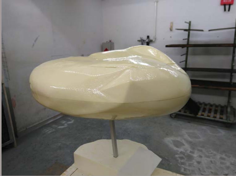
The two-component epoxy resin was applied in multiple layers until the desired layer thickness of 3–4mm was reached.
