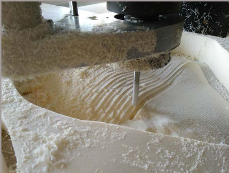
Each layer was cut by a CNC milling machine from Styrodur.
