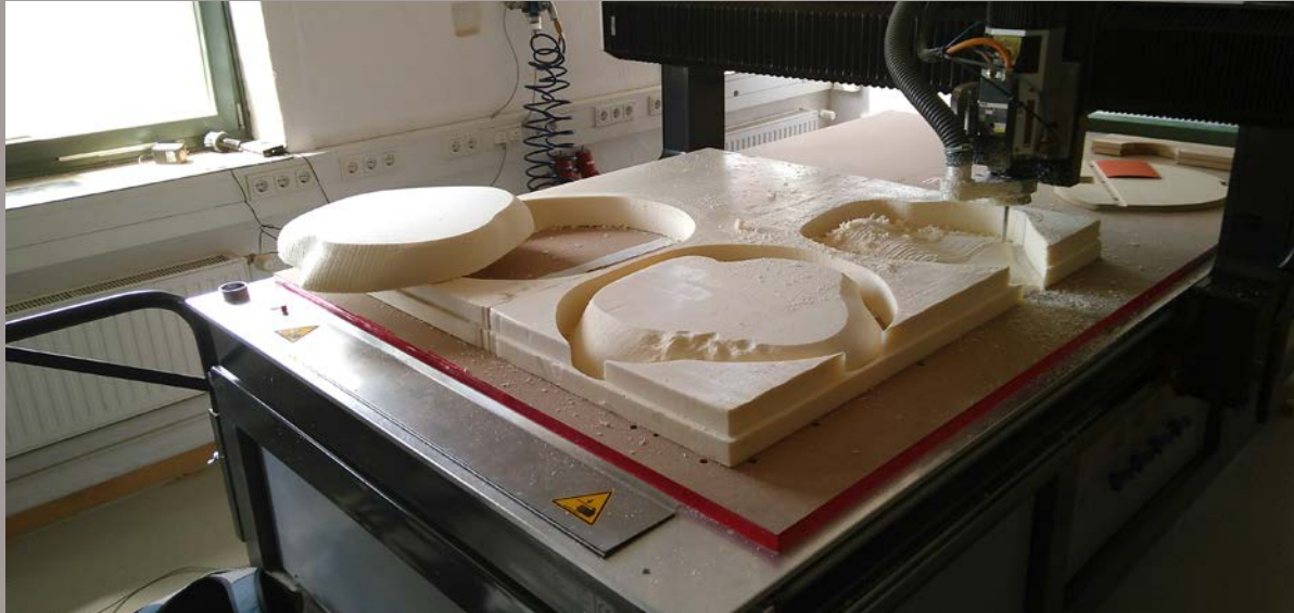
The positive mold was designed and planned in a 3D software and separated in four layers.
