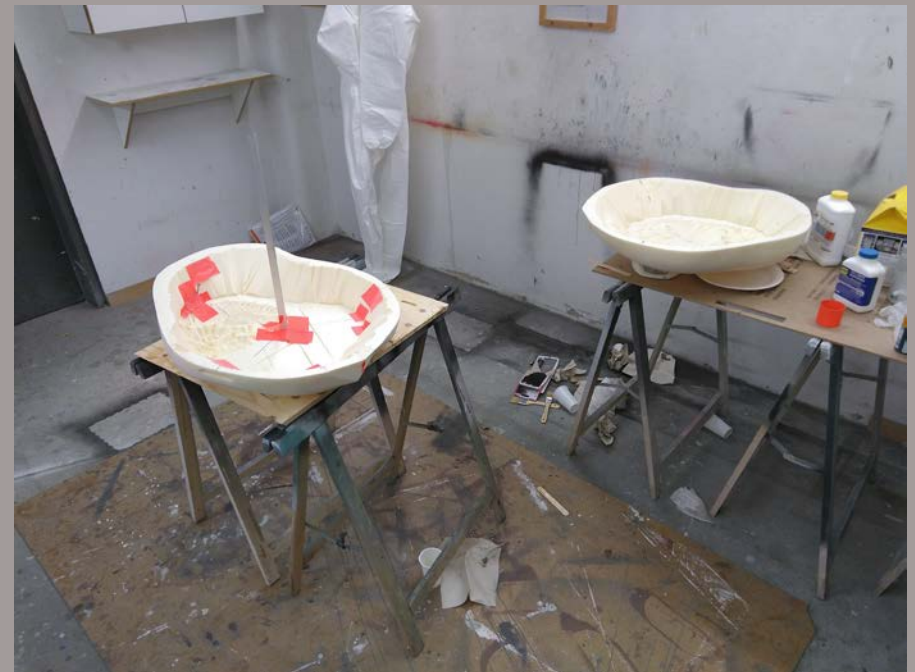
The four layers were scooped out by hand to save material and glued together to create the final shape of the positive mold.
