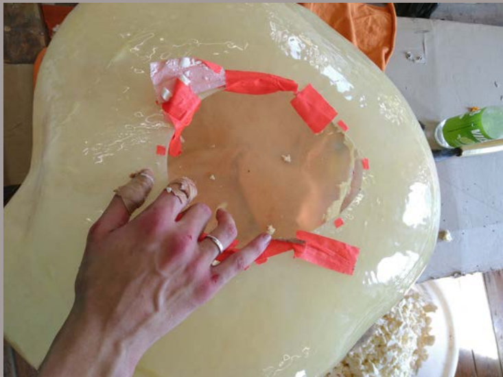
To remove the Polystyrol an opening at the bottom had to be cut and the material had to be removed by hand.
